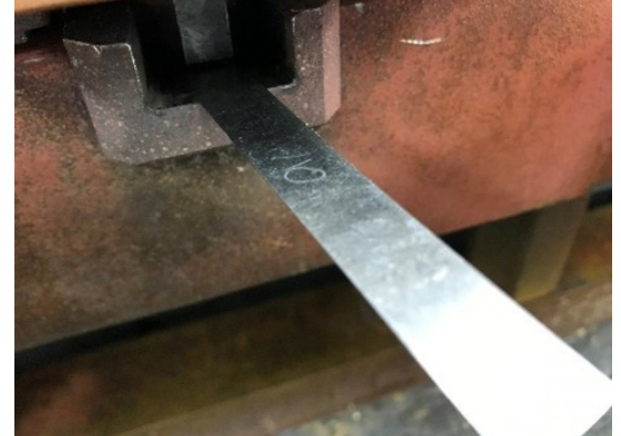
Image #4: Feeler gage being used to assess gap between guide and mold slide.
