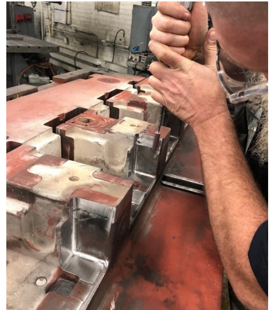
Image #5: Mold being "hot fitted" by AG Journeyman Patternmaker
